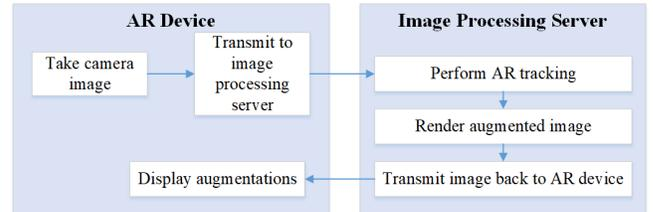
Fig. 3: AR system model with offloaded processing [7]
