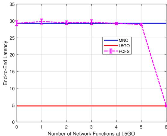
Fig. 20: Average AR packet latency under FCFS algorithm
