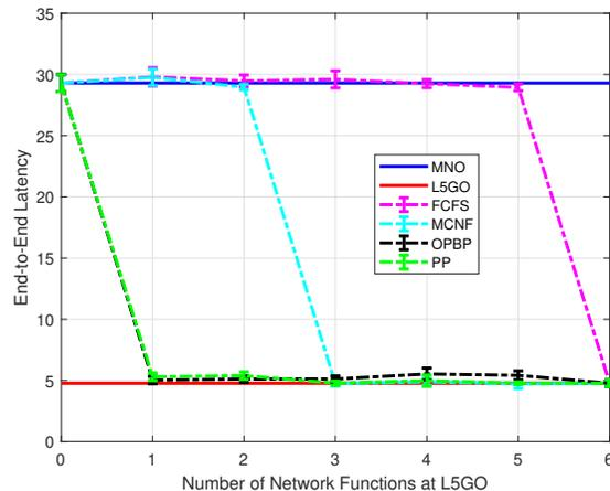
Fig. 24: Average packet latency of AR use case
