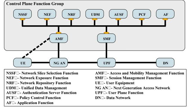
Fig. 1: Service based representation of 5G architecture [12]
