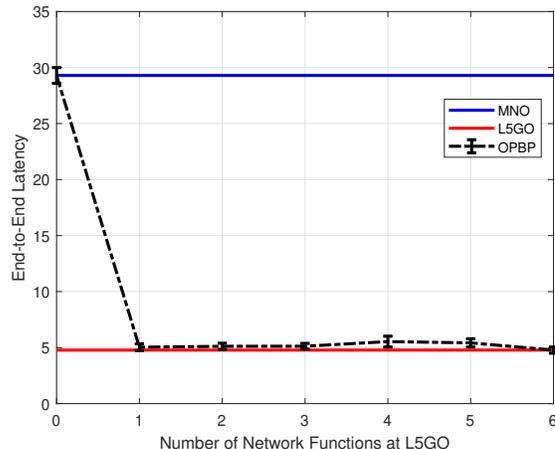
Fig. 22: Average AR packet latency under OPBP algorithm
