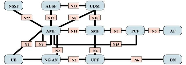
Fig. 2: Reference point representation of 5G architecture [12]
