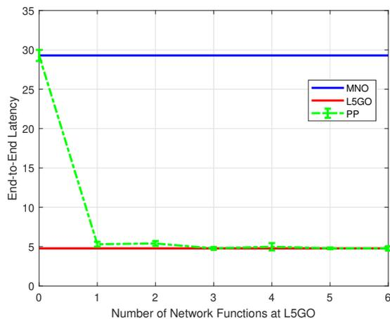
Fig. 23: Average AR packet latency under PP algorithm
