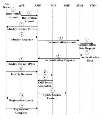
Fig. 7: Message sequence chart for AR device registration procedure
