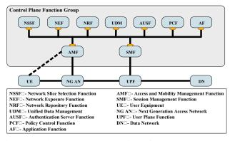
Fig. 1: Service based representation of 5G architecture [12]
