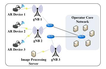
Fig. 4: An AR network with terminal devices and the AR server
