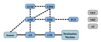
Fig. 11: Architectural components of L5GO to serve the massive wireless sensor networks use case
