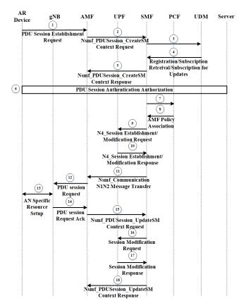
Fig. 8: Message sequence chart for session establishment between AR device and server
