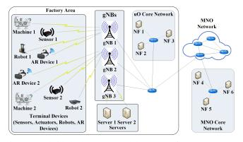
Fig. 19: Hybrid deployment model to serve factory use cases
