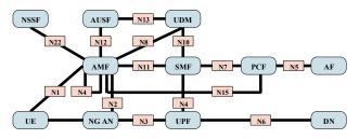
Fig. 2: Reference point representation of 5G architecture [12]
