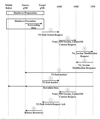
Fig. 12: Message sequence chart for handover procedure of robots
