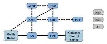
Fig. 13: Architectural components of L5GO to serve the mobile robots use case
