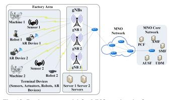
Fig. 18: Deployment model for MNO serving the factory use cases
