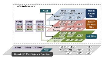
Fig. 14: Proposed architecture of L5GO with three network slices
