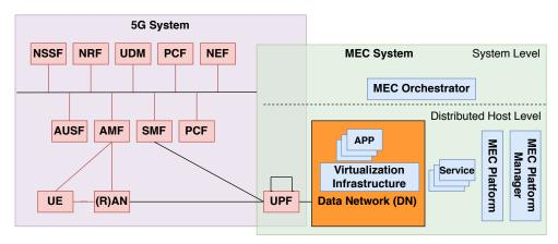
Fig. 13: Integrated MEC Deployment in 5G Network [131].
