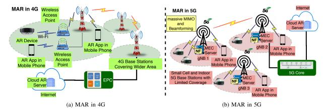
Fig. 11: Comparison of Network Architectures for MAR.
