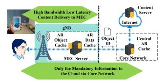
Fig. 14: A Mobile Augmented Reality Service Scenario [42].
