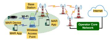
Fig. 8: Localized System Architecture for a MAR System using only MAR Devices.
